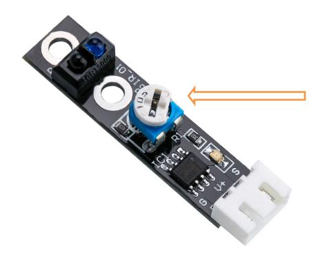
The component which is pointed at is potentiometer. It can adjust the sensitivity of the line tracking module by change its resistance value.
