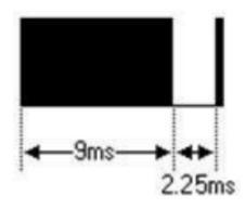
Note: After impulse waveform enters into integration of sensor, owing to the fact that integration of sensor should be decoded, signal magnified and plastic, you should note the time when there are no infrared signals, its output terminal is high level, is low level when there are signals. So the level of output signal is opposite to transmitting terminal. Everybody can see receiver pulse through oscilloscope, understand program with wave form seen.
