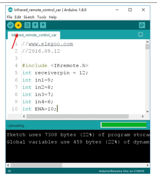
When done uploading, disconnecting the car to the computer. Then turn on the power switch and put the car on the ground. Press the button on the remote and you can see the car move accordingly as you command.
