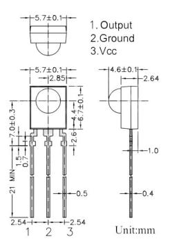
The connection of receiver module is as below:
