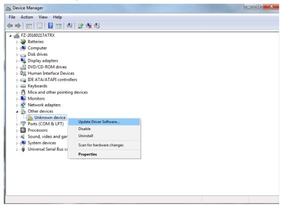
It shows that the driver has not been installed, and you need to click Browse my computer for driver software to find the drivers. The drives is in the Arduino folder. Normally you will install the folder in C:\Program Files (x86)\Arduino.
